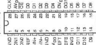
DW D1PW PACKAGE (TOP VIEW)
